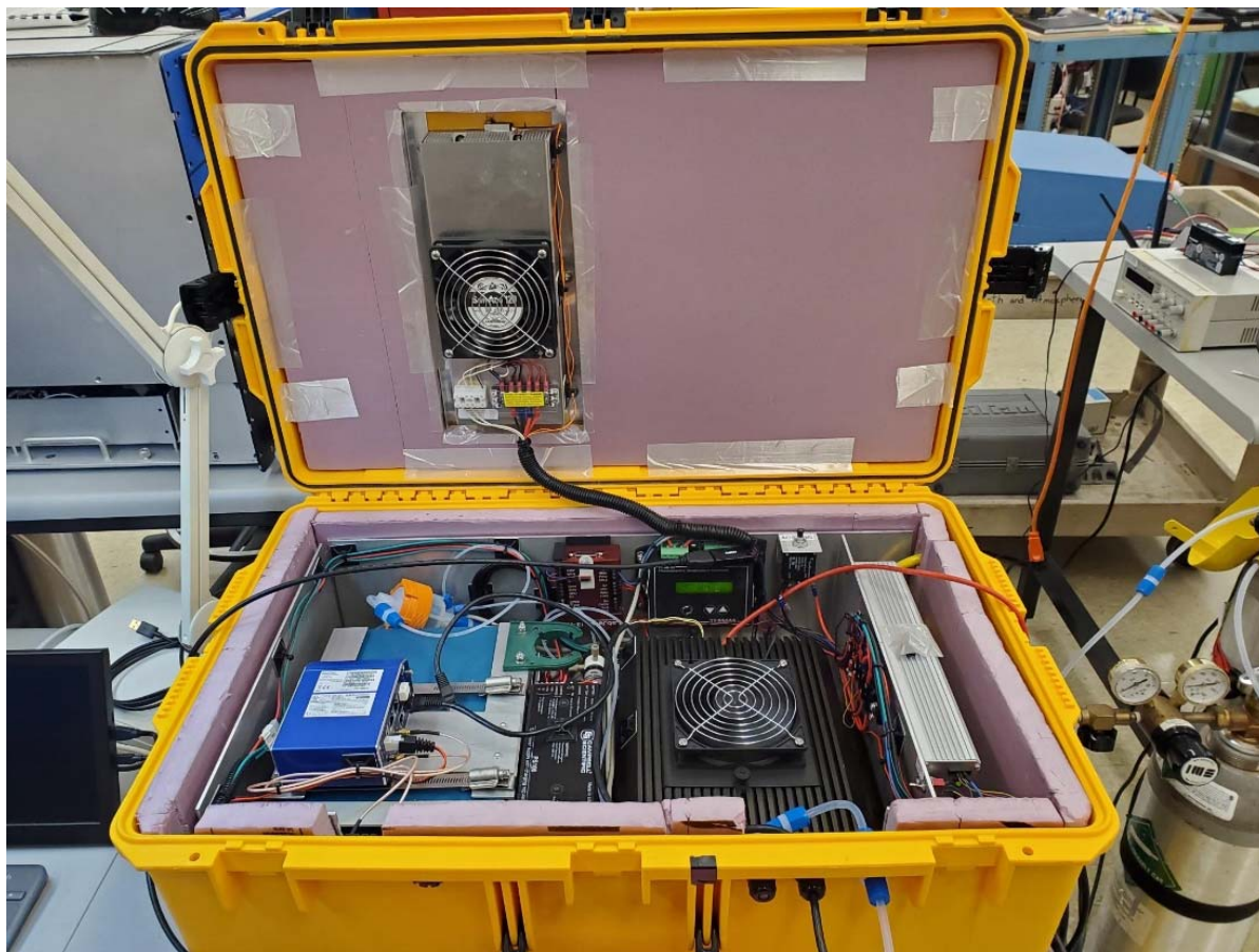
Figure 67. Instrumented weatherproof enclosure installed on the two commercial boats showing the 2B Tech O 3 monitor (blue box, bottom left), dual-sim cellular router (small blue box above 2B), backup battery (black box, center), zeroing cartridge (orange and clear, left rear), rugged industrial computer (black box with fan on top, right), high efficiency 24VDC power supply (silver box, far right). The rear panel of the chassis provides space for the LabJack U3 data card (red, center rear), thermoelectric temperature controller (black with green screen, rear behind computer), and circuit breaker for the thermoelectric cooler system (black button on silver tab, right of temperature controller). Space for mounting the NO 2 photocells is reserved on top of the O 3 analyzer, near the cellular router and will be installed for future campaigns.
